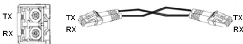
Figure 10 Cable Connection of Gigabit SFP Optical Module
